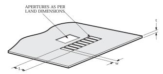
Figure 14. Solder stencil aperature.
