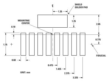
Figure 13. Stencil and PCBA.
