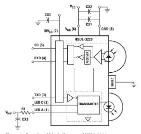
Figure 1. Functional block diagram of HSDL-3220.
