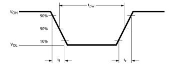
Figure 5. RxD output waveform.
