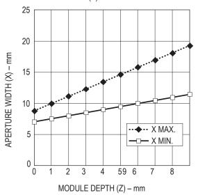
Figure 20. Aperture width (X) vs. module depth.
