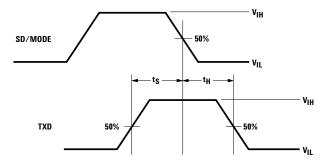
Figure 4. Bandwidth selection timing at FIR mode.
