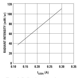
Figure 9. Radiant Intensity vs  $I_{LEDA}$ .
