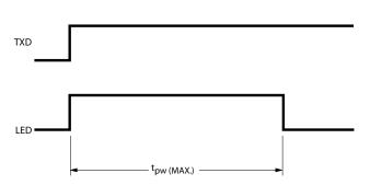
Figure 7. TxD "Stuck On" protection waveform.
