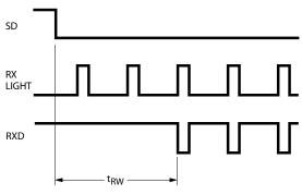
Figure 8. Receiver wakeup time waveform.
