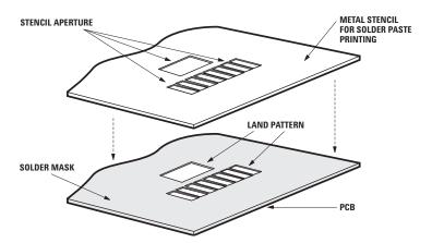
Figure 12. Stencil and PCBA.
