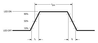
Figure 6. LED optical waveform.
