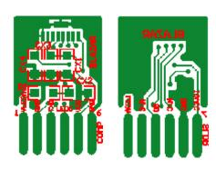
Figure 16. PCB layout suggestion.
