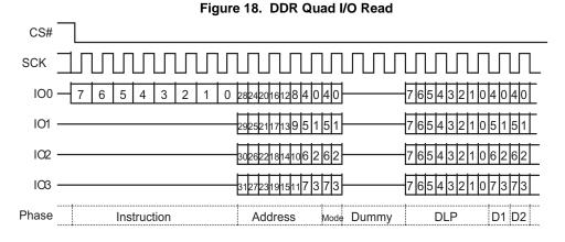
Additional sequence diagrams, specific to each command, are provided in Section 9., Commands on page 60.
