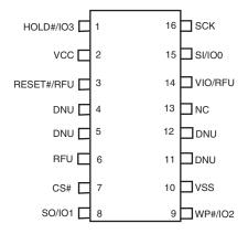
Figure 39. 16-Lead SOIC Package, Top View
