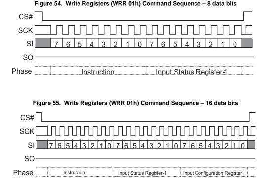
The Write Registers (WRR) command allows the user to change the values of the Block Protect (BP2, BP1, and BP0) bits to define the size of the area that is to be treated as read-only. The Write Registers (WRR) command also allows the user to set the Status Register Write Disable (SRWD) bit to a 1 or a 0. The Status Register Write Disable (SRWD) bit and Write Protect (WP#) signal allow the BP bits to be hardware protected.
