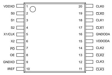
Figure 2. Pin Configuration (Top View)
