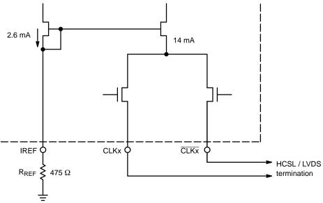
**Figure 6. Simplified Output Structure**
