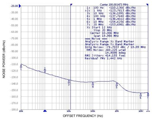
Figure 3. Typical Phase Noise Plot at 100 MHz; (f<sub>CLKIN</sub> = 25 MHz Crystal , f<sub>CLKOUT</sub> = 100 MHz SS OFF, RMS Phase Jitter for Integration Range 12 kHz to 20 MHz = 414 fs, Output Termination = HCSL type)
