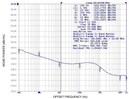
Figure 4. Typical Phase Noise Plot at 200 MHz; (f<sub>CLKIN</sub> = 25 MHz Crystal , f<sub>CLKOUT</sub> = 200 MHz SS OFF, RMS Phase Jitter for Integration Range 12 kHz to 20 MHz = 406 fs, Output Termination = HCSL type)
