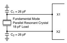
Figure 5. Crystal Interface Loading
