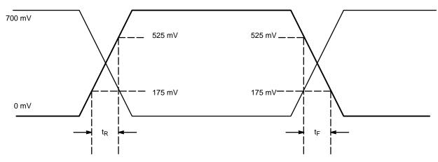
Figure 9. HCSL Output Parameter Characteristics
