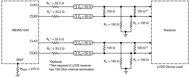
Figure 8. Typical Termination for LVDS Device Load
