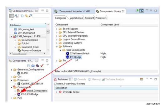
2. Double-click LVHBridge component in the Components window to show the configuration in the Component Inspector view.
