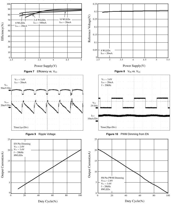
Figure 11 Enable Pin Dimming
