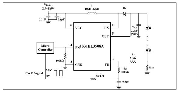
Figure 6 Constant output current with PWM dimming control
