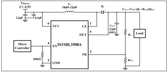
Figure 4 Constant output voltage for general purpose use
