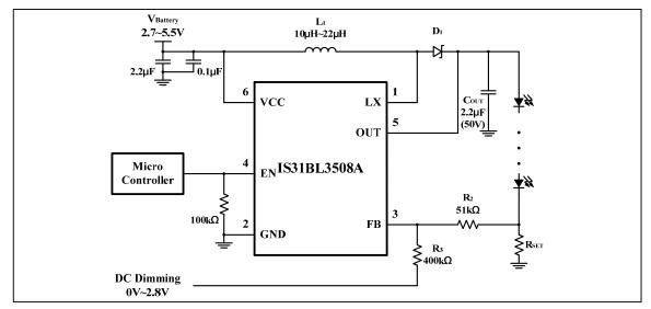
Figure 5 Constant output current with DC dimming input
