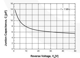
Figure 7. Typical Junction Capacitance
