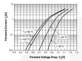
Figure 3. Typical Instantaneous Forward Characteristics
