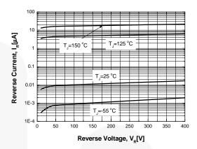
Figure 4. Typical Reverse Characteristics
