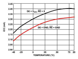
FIGURE 12. SUPPLY CURRENT vs TEMPERATURE
