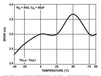
FIGURE 19. DRIVER DIFFERENTIAL SKEW vs TEMPERATURE (ISL32475E)
