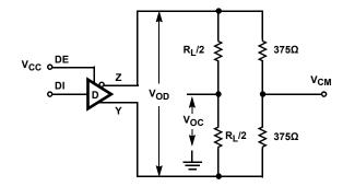
FIGURE 3B.  $V_{\mbox{\scriptsize OD}}$  and  $V_{\mbox{\scriptsize OC}}$  with common mode load
