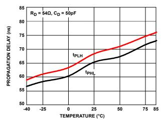
FIGURE 18. DRIVER DIFFERENTIAL PROPAGATION DELAY vs TEMPERATURE (ISL32475E)
