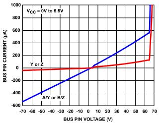
FIGURE 15. BUS PIN CURRENT vs BUS PIN VOLTAGE
