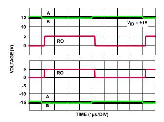
FIGURE 22. RECEIVER PERFORMANCE WITH ±15V CMV (ISL32470E, ISL32472E)
