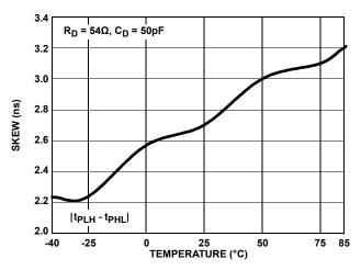
FIGURE 21. DRIVER DIFFERENTIAL SKEW vs TEMPERATURE (ISL32478E)
