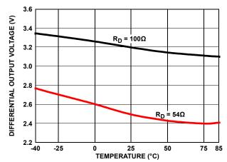
FIGURE 11. DRIVER DIFFERENTIAL OUTPUT VOLTAGE vs
