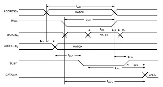
Figure 12. Write Timing with Busy Input ( $M/\overline{S} = LOW$ )
