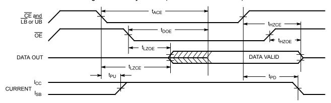
Figure 6. Read Cycle No. 3 (Either Port) [21, 23, 24, 25]
