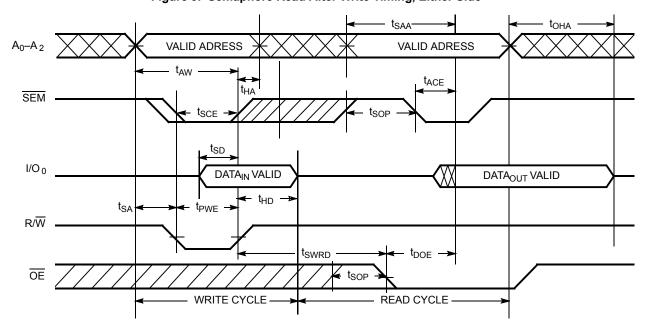
Figure 10. Timing Diagram of Semaphore Contention  $^{[36,\ 37,\ 38]}$
