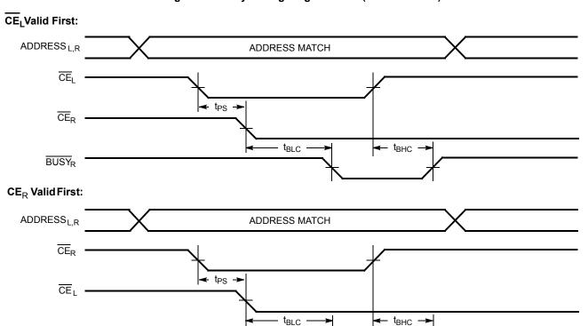
Figure 14. Busy Timing Diagram No. 2 (Address Arbitration)  $^{[40]}$
