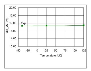
Figure 51: V<sub>CCUV-</sub> vs. temperature
