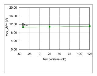
Figure 50: V<sub>CCUV+</sub> vs. temperature
