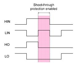
Figure 9: Illustration of shoot-through protection circuitry
