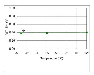
Figure 55: V<sub>IT,TH-</sub> vs. temperature
