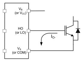
Figure 2: HVIC sinking current
