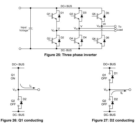
Also when the V phase current flows from the inductive load back to the inverter (see Figures 28 and 29), and Q4 IGBT switches on, the current commutation occurs from D3 to Q4. At the same instance, the voltage node,  $V_{S2}$ , swings from the positive DC bus voltage to the negative DC bus voltage.
