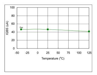
Figure 49: I<sub>QBS</sub> vs. temperature
