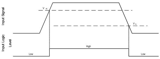
Figure 7: HIN & LIN input thresholds
