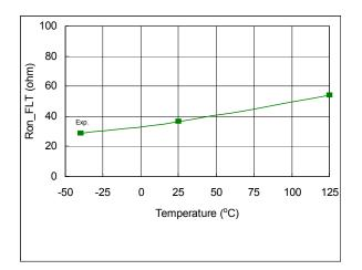
Figure 47: R<sub>ON,FLT</sub> vs. temperature
