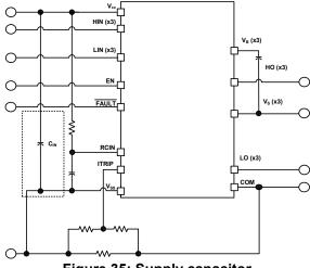
Figure 35: Supply capacitor
