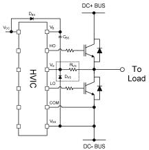
Figure 37: V<sub>s</sub> clamping diode
