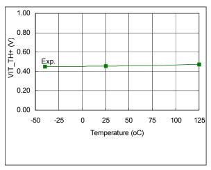
Figure 54: VIT,TH+ vs. temperature
