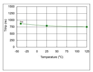
Figure 43: t<sub>ITRIP</sub> vs. temperature
