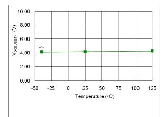
Figure 59: V<sub>DCBUSSTH-</sub> vs. temperature
