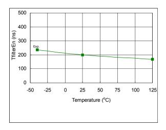
Figure 45  $t_{EN}$  vs. temperature
