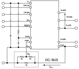
Figure 13: Programming the over-current protection
