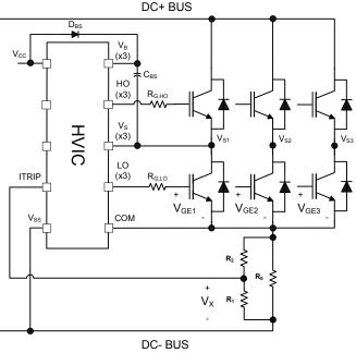
Figure 24: Separate V<sub>ss</sub> and COM pins
