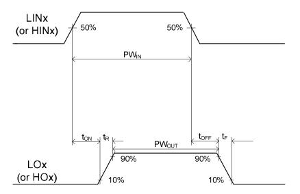
Figure 3: Switching time waveforms
