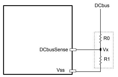
Figure 16: Programming the DC bus over-voltage protection
