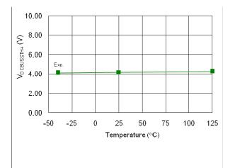
Figure 58: V<sub>DCBUSSTH+</sub> vs. temperature
