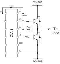
Figure 36: V<sub>S</sub> resistor
