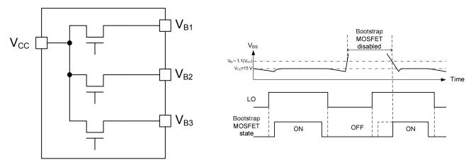
Figure 22: Internal bootstrap MOSFET connection
