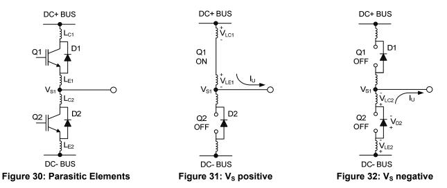
In a typical motor drive system, dV/dt is typically designed to be in the range of 3-5 V/ns. The negative V<sub>S</sub> transient voltage can exceed this range during some events such as short circuit and over-current shutdown, when di/dt is greater than in normal operation.
