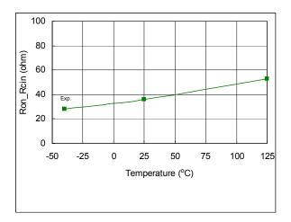
Figure 46: R<sub>ON,RCIN</sub> vs. temperature
