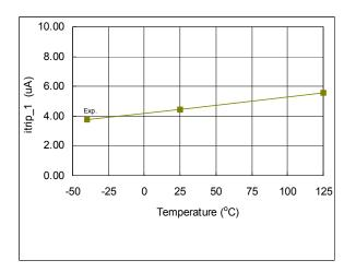
Figure 60: IITRIP+ vs. temperature
