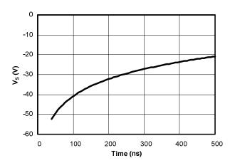
Figure 33: Negative V<sub>s</sub> transient results for an International Rectifier HVIC
