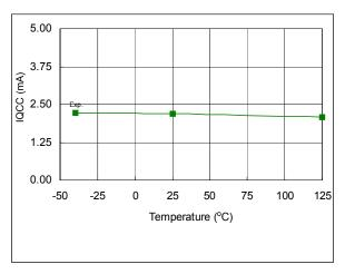
Figure 48: I<sub>QCC</sub> vs. temperature
