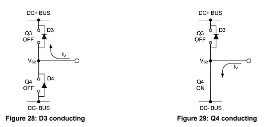
However, in a real inverter circuit, the  $V_S$  voltage swing does not stop at the level of the negative DC bus, rather it swings below the level of the negative DC bus. This undershoot voltage is called "negative  $V_S$  transient".
