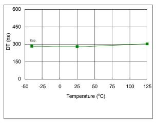
Figure 42: DT vs. temperature
