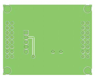
Figure 5: Evaluation Board Solder Side Layout.
