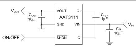
Figure 6: Typical Charge Pump Boost Converter Circuit.
