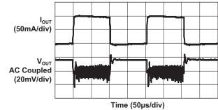
Output Ripple (I<sub>OUT</sub> = 100mA; V<sub>IN</sub> = 2.5V)
