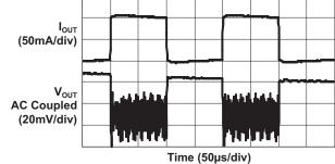
**Output Ripple** (I<sub>OUT</sub> = 100mA; V<sub>IN</sub> = 3.0V)
