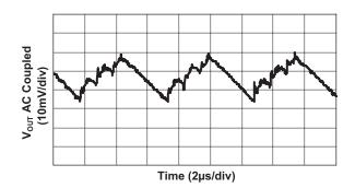
Load Transient Response (V<sub>IN</sub> = 2.6V)
