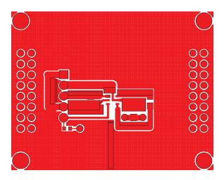
Figure 4: Evaluation Board Component Side Layout.
