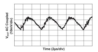
Load Transient Response (V<sub>IN</sub> = 2.4V)
