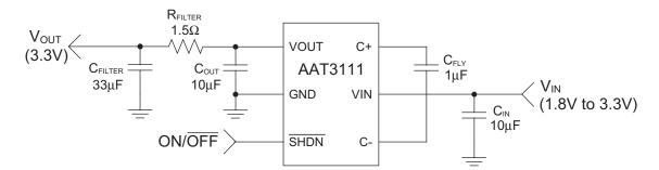
Figure 2: Application With Output Ripple Reduction Filter.
