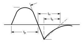
Figure 15. Diode Reverse Recovery Waveform
