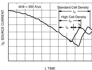
Figure 11. Reverse Recovery Time (t<sub>rr</sub>)
