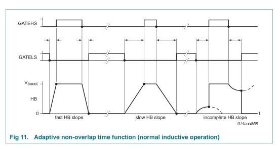
The non-overlap time depends on the HB slope but it has upper and lower limits.
