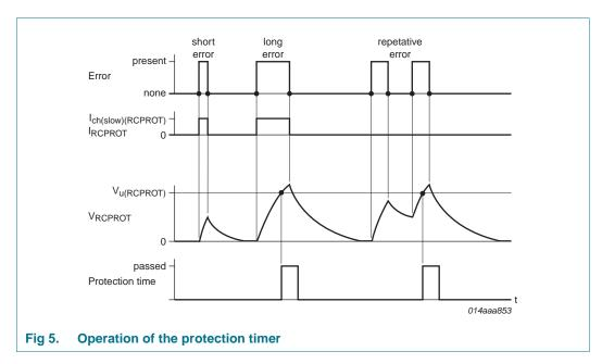
Figure 5 shows the operation of the protection timer. When an error condition occurs, a fixed current  $I_{ch(slow)(RCPROT)}$  (100  $\mu$ A) flows from the RCPROT pin and charges  $C_{prot}$ .  $R_{prot}$  causes the voltage to increase exponentially. The protection time elapses when the voltage on the RCPROT pin reaches the upper switching level  $V_{u(RCPROT)}$  (4 V). When the protection time has elapsed, the appropriate protective action is taken and  $C_{prot}$  is discharged.
