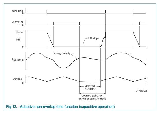
The MOSFET is forced to switch on when the half-bridge slope fails to start and the oscillator voltage reaches  $V_{u(CFMIN)}$ .
