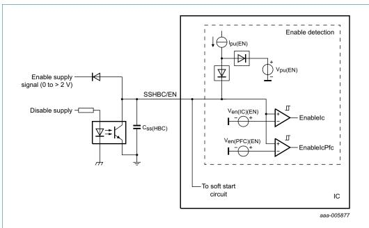
Fig 4. Circuit configuration around the SSHBC/EN pin
