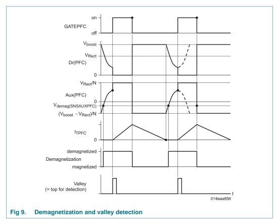
The valley sensing block connected to the SNSAUXPFC pin detects the valleys. This block measures the PFC transformer auxiliary winding voltage, which is a reduced and inverted copy of the MOSFET drain voltage. When a valley of the drain voltage (= top at SNSAUXPFC voltage) is detected, the MOSFET is switched on.
