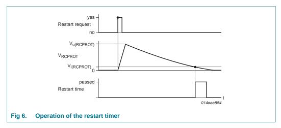
Figure 6 shows the operation of the restart timer. Normally  $C_{prot}$  is discharged to 0 V. When a restart is requested,  $C_{prot}$  is quickly charged to the upper switching level  $V_{u(RCPROT)}$ . Then the RCPROT pin becomes high ohmic and  $C_{prot}$  discharges through  $R_{prot}$ . The restart time has elapsed when  $V_{RCPROT}$  reaches the lower switching level  $V_{l(RCPROT)}$  (0.5 V). The IC restarts and  $C_{prot}$  is discharged.
