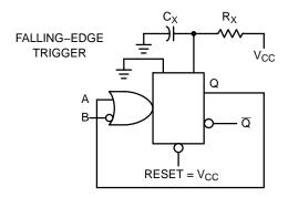
Figure 14. Non-retriggerable Monostable Circuitry
