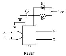
Figure 12. Discharge Protection During Power Down
