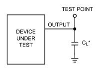
\*Includes all probe and jig capacitance
