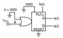
Figure 15. Connection of Unused Section
