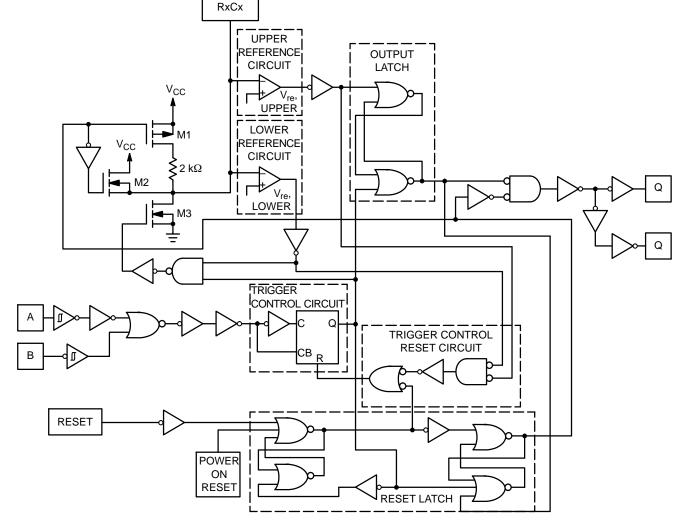
Figure 10. Logic Detail (1/2 the Device)
