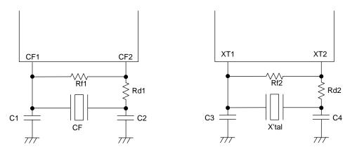
Figure 1 Ceramic Oscillation Circuit
