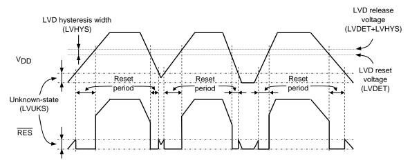
Figure 9 Waveform observed when both POR and LVD functions are used (RESET pin: Pull-up resistor RRES only)
