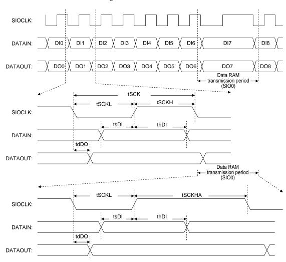
Figure 6 Serial I/O Output Waveforms
