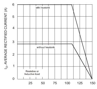
T<sub>C</sub>, CASE TEMPERATURE (°C) Fig. 1 Forward Current Derating Curve
