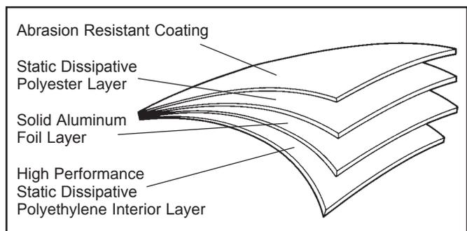
Figure 3. Statshield® Foil (EMI/RFI) MBB Bag Layer construction
