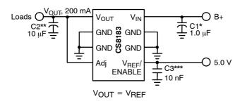
Figure 7. Tracking Regulator at the Same Voltage
