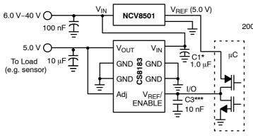
Figure 11. Alternative ENABLE Circuit
