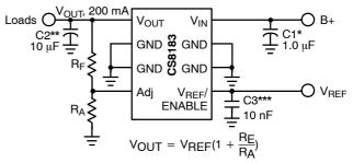
Figure 8. Tracking Regulator at Higher Voltages
