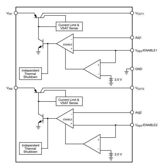
Figure 1. Block Diagram
