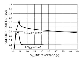
Figure 3. Quiescent Current vs. Input Voltage (Operating Mode)
