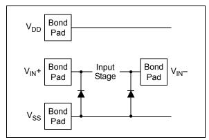
FIGURE 4-4: Simplified Analog Input ESD Structures.
