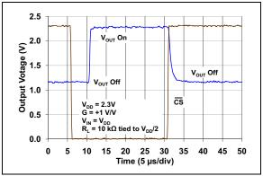
**FIGURE 2-55:** Chip Select Voltage, Output Voltage vs. Time with  $V_{DD} = 2.3V$ .
