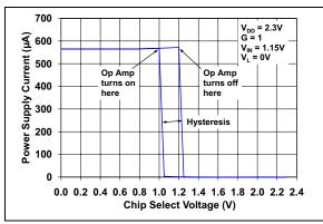
**FIGURE 2-52:** Power Supply Current vs. Chip Select Voltage with  $V_{DD} = 2.3V$ .
