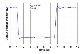
FIGURE 2-46: Inverting Small Signal Step Response.
