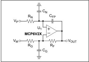
FIGURE 4-10: Amplifier with Parasitic Capacitance.
