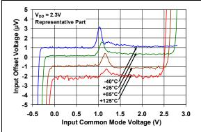
**FIGURE 2-7:** Input Offset Voltage vs. Common Mode Voltage with  $V_{DD} = 2.3V$ .
