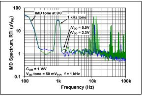
**FIGURE 2-38:** Intermodulation Distortion vs. Frequency with V<sub>DD</sub> Disturbance (see Figure 1-7).
