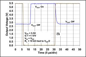
**FIGURE 2-56:** Chip Select Voltage, Output Voltage vs. Time with  $V_{DD} = 5.5V$ .
