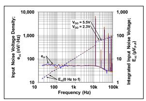
**FIGURE 2-35:** Input Noise Voltage Density and Integrated Input Noise Voltage vs. Frequency.
