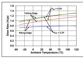
FIGURE 2-48: Slew Rate vs. Ambient Temperature.
