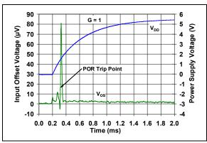
**FIGURE 2-42:** Input Offset Voltage vs. Time at Power Up.
