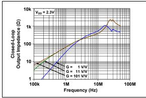
**FIGURE 2-31:** Closed-Loop Output Impedance vs. Frequency with  $V_{DD} = 2.3V$ .
