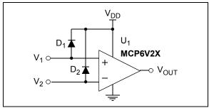
**FIGURE 4-5:** Protecting the Analog Inputs Against High Voltages.
