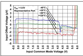
**FIGURE 2-8:** Input Offset Voltage vs. Common Mode Voltage with  $V_{DD} = 5.5V$ .
