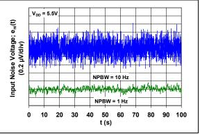
**FIGURE 2-40:** Input Noise vs. Time with 1 Hz and 10 Hz Filters and  $V_{DD} = 5.5V$ .
