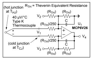
**FIGURE 4-15:** Thermocouple Sensor; Simplified Circuit.
