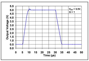
FIGURE 2-45: Non-inverting Large Signal Step Response.
