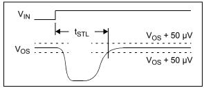
**FIGURE 1-2:** Offset Correction Settling Time.
