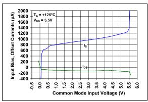
**FIGURE 2-15:** Input Bias and Offset Currents vs. Common Mode Input Voltage with  $T_A = +125$ °C.
