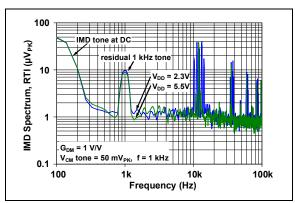
**FIGURE 2-37:** Intermodulation Distortion vs. Frequency with V<sub>CM</sub> Disturbance (see Figure 1-7).
