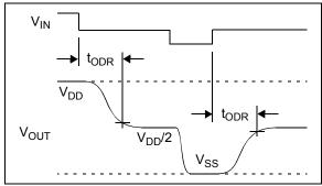
FIGURE 1-3: Output Overdrive Recovery.
