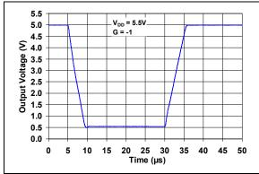
**FIGURE 2-47:** Inverting Large Signal Step Response.
