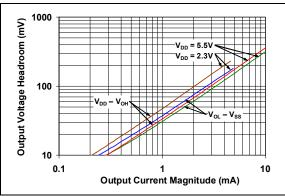
FIGURE 2-19: Output Voltage Headroom vs. Output Current.
