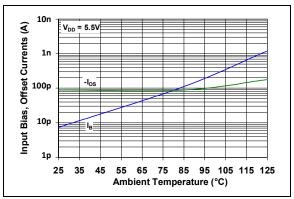
**FIGURE 2-16:** Input Bias and Offset Currents vs. Ambient Temperature with  $V_{DD} = +5.5V$ .
