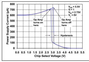
**FIGURE 2-53:** Power Supply Current vs. Chip Select Voltage with  $V_{DD} = 5.5V$ .
