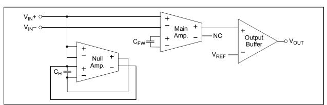
**FIGURE 4-3:** Auto-zeroing Mode of Operation  $(\phi_2)$ ; Equivalent Diagram.
