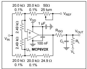
FIGURE 1-7: Test Circuit for Dynamic Input Behavior.
