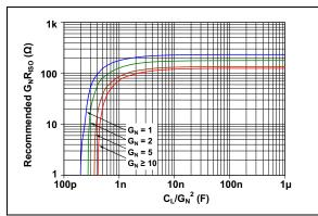
**FIGURE 4-8:** Recommended R<sub>ISO</sub> values for Capacitive Loads.
