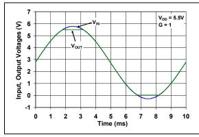
FIGURE 2-43: The MCP6V26/7/8 Device Shows No Input Phase Reversal with Overdrive.
