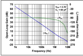
**FIGURE 2-26:** Open-Loop Gain vs. Frequency with  $V_{DD} = 2.3V$ .
