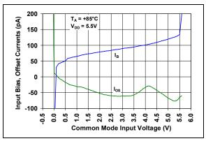
**FIGURE 2-14:** Input Bias and Offset Currents vs. Common Mode Input Voltage with  $T_A = +85$ °C.
