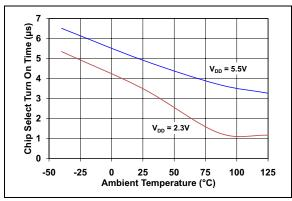
**FIGURE 2-59:** Chip Select Turn On Time vs. Ambient Temperature.
