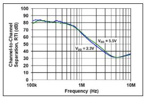
**FIGURE 2-33:** Channel-to-Channel Separation vs. Frequency.
