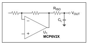
**FIGURE 4-7:** Output Resistor, R<sub>ISO</sub>, Stabilizes Capacitive Loads.
