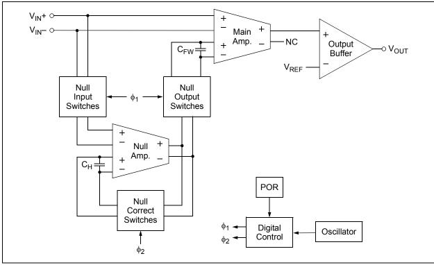
FIGURE 4-1: Simplified Auto-Zeroed Op Amp Functional Diagram.
