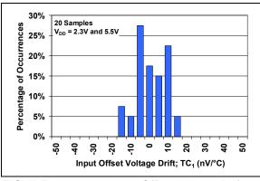
FIGURE 2-2: Input Offset Voltage Drift.
