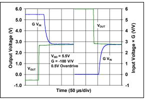
**FIGURE 2-49:** Output Overdrive Recovery vs. Time with G = -100 V/V.
