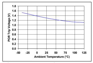
**FIGURE 2-24:** Power On Reset Voltage vs. Ambient Temperature.
