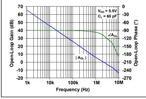
**FIGURE 2-27:** Open-Loop Gain vs. Frequency with  $V_{DD} = 5.5V$ .
