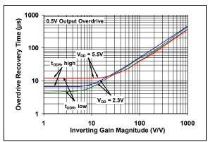
**FIGURE 2-50:** Output Overdrive Recovery Time vs. Inverting Gain.
