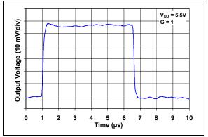
FIGURE 2-44: Non-inverting Small Signal Step Response.
