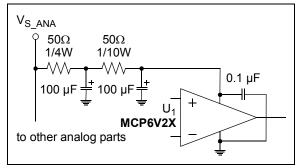
FIGURE 4-11: Additional Supply Filtering.
