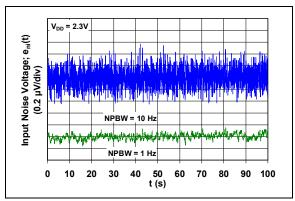
**FIGURE 2-39:** Input Noise vs. Time with 1 Hz and 10 Hz Filters and  $V_{DD} = 2.3V$ .
