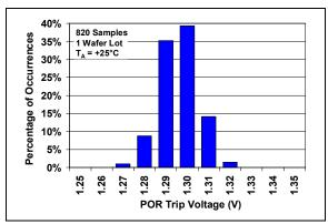
**FIGURE 2-23:** Power On Reset Trip Voltage.
