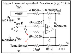
FIGURE 4-16: Thermocouple Sensor.
