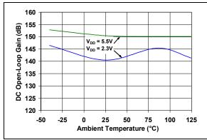
**FIGURE 2-13:** DC Open-Loop Gain vs. Ambient Temperature.
