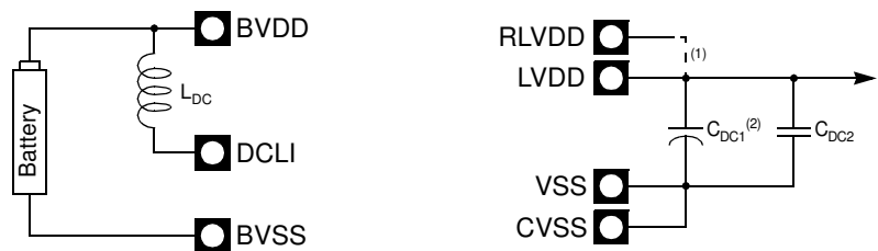
Figure 135. Battery DC-DC Connection
