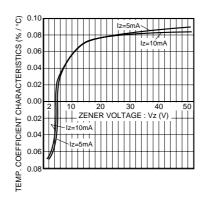
Fig.3 Zener voltagetemp.coefficient characteristics
