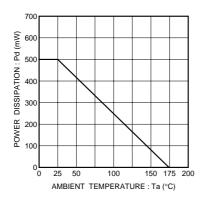
Fig. 2 Derating curve
