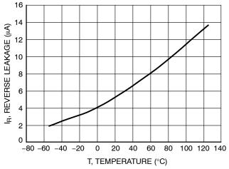
Figure 2. Reverse Leakage versus Temperature
