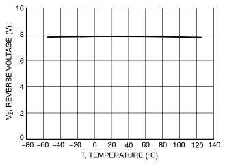
Figure 1. Reverse Voltage versus Temperature
