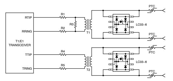
Figure 7. Typical T1 Line Card Protection
