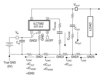
Figure 7. Effects of Poor Circuit Layout
