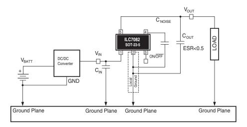
Figure 8. Recommended Application Circuit Schematic
