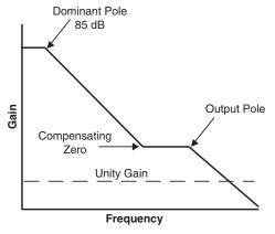
Figure 1. ILC7082 RF LDO Frequency Response
