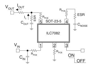
Figure 6. Inherent PCB resistance
