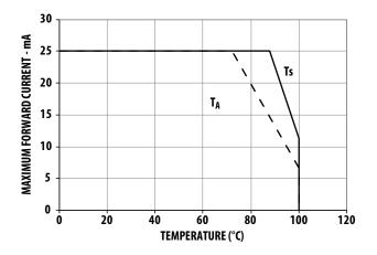
Maximum forward current graphs based on ambient temperature,  $T_A$  are with reference to thermal resistance  $R_{\theta J-A}$  as follows. For more details, see Precautionary Notes (4).
