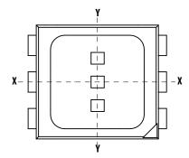
**Figure 14 Recommended Soldering Land Pattern**
