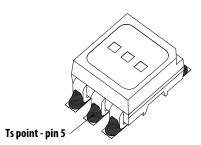
$T_S$  can be measured easily by mounting a thermocouple on the soldering joint as shown in preceding illustration, while  $R_{\theta J-S}$  is provided in the data sheet. Customers should verify the  $T_S$  of the LED in the final product to ensure that the LEDs are operated within all maximum ratings stated in the data sheet.
