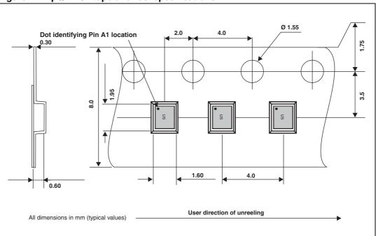
Figure 17. µQFN-8L tape and reel specifications
