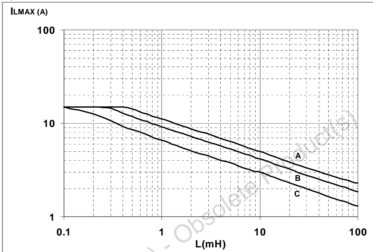
Figure 26. SO-16L Maximum turn off current versus load inductance
