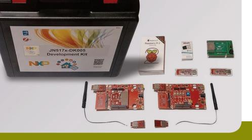
For ZigBee® 3.0 Smart Home and Lighting mesh networks with NFC
