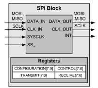
SPI configuration register (SPI\_CFG) sets master/slave functionality, clock speed and interrupt select. SPI control register (SPI\_CR) provides four control bits and four status bits for device interfacing and synchronization.
