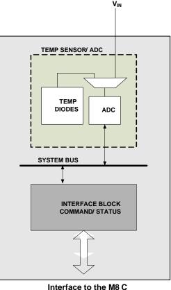
Figure 1. ADC System Performance Block Diagram
