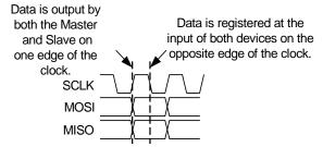
A device can be a master or slave. A master outputs clock and data to the slave device and inputs slave data. A slave device inputs clock and data from the master device and outputs data for input to the master. Together, the master and slave are essentially a circular Shift register, where the master generates the clocking and initiates data transfers.
