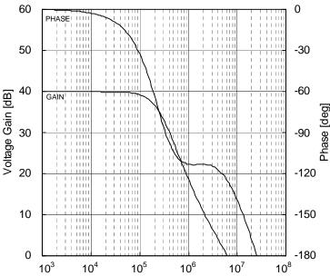
$\label{eq:figure 23.} Figure 23. \\ Voltage Gain, Phase vs Frequency \\ (VCC/VEE=+15V/-15V, Av=40dB, R_L=2k\Omega, T_A=25^{\circ}C)$
