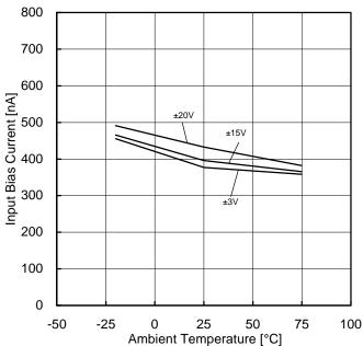
Figure 13. Input Bias Current - Ambient Temperature  $(V_{ICM}=0V, E_k=0V)$
