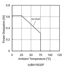
6.2 mW/°C When using the unit above T<sub>A</sub>=25°C, subtract the value above per Celsius degree.
