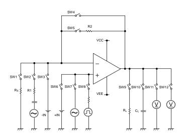
Figure 25. Test Circuit 2 (each Op-Amp)
