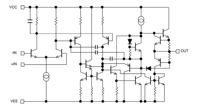
Figure 1. Simplified Schematic (1channel only)
