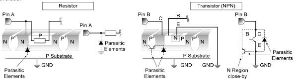
Figure 32. Example of monolithic IC structure
