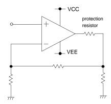
Figure 34. The Example of Output Short Protection
