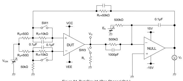
Figure 24. Test Circuit1 (One Channel Only)
