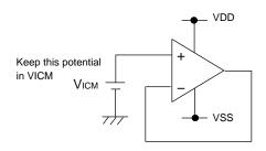
Figure 33. Example of Application Circuit for Unused Op-amp
