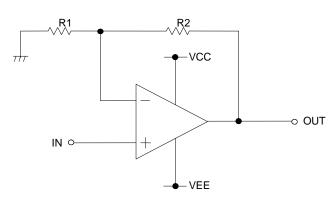
Figure 31. Non-inverting Amplifier Circuit
