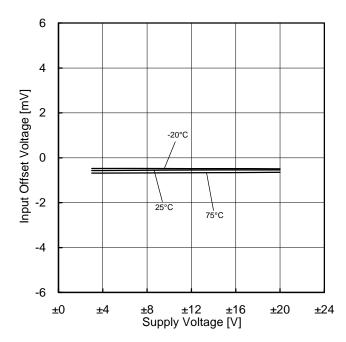
$\begin{array}{c} Figure \ 10. \\ Input \ Offset \ Voltage \ - \ Supply \ Voltage \\ (V_{ICM}{=}0V, \ E_k{=}0V) \end{array}$
