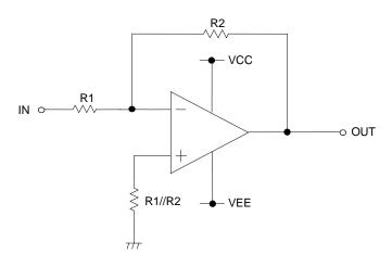
Figure 30. Inverting Amplifier Circuit
