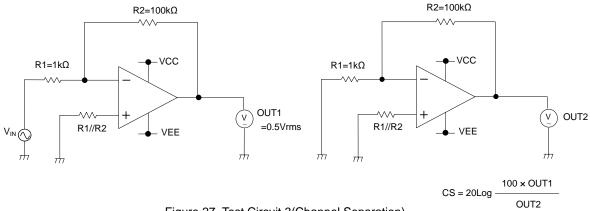
Figure 27. Test Circuit 3(Channel Separation)
