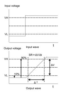
Figure 26. Slew Rate Input Waveform
