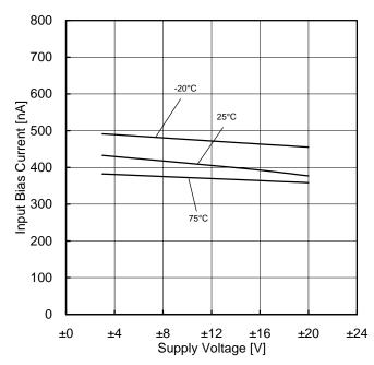
Figure 12. Input Bias Current - Supply Voltage ( $V_{\text{ICM}}$ =0V,  $E_k$ =0V)
