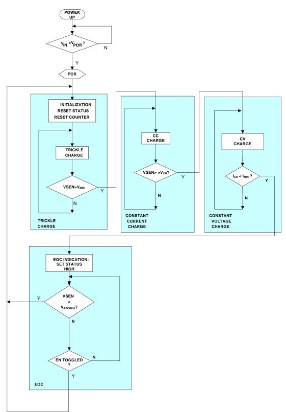
FIGURE 17. CHARGING STATE DIAGRAM
