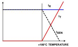
FIGURE 21. CURRENT SIGNALS AT THE AMPLIFIER CA INPUT
