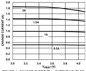
FIGURE 4. CHARGE CURRENT vs OUTPUT VOLTAGE
