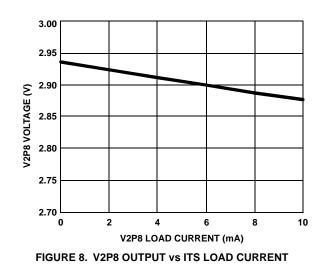
**Typical Operating Performance** The test conditions for the Typical Operating Performance are:  $V_{IN} = 5V$ ,  $T_A = +25^{\circ}C$ ,
