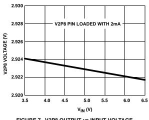
FIGURE 7. V2P8 OUTPUT vs INPUT VOLTAGE
