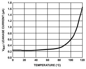
FIGURE 11. REVERSE CURRENT vs TEMPERATURE
