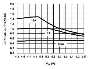
FIGURE 6. CHARGE CURRENT vs INPUT VOLTAGE
