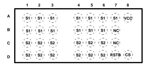
TOP VIEW Figure 2. Pin Functions
