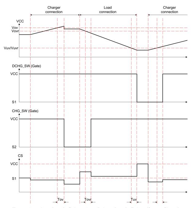
Figure 6. Over-charge Detection/Release, Over-discharge Detection/Release (Connect Charger)
