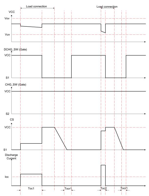
Figure 8. Discharge Over-Current Detection1, Discharge Over-current Detection2 (Short Circuit)
