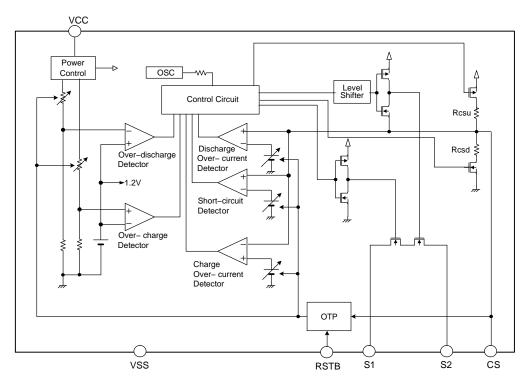
Figure 3. Block Diagram
