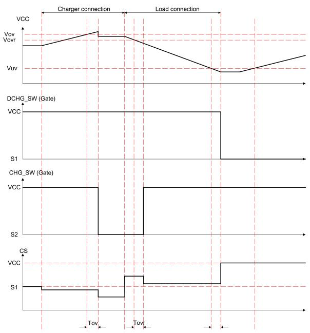
Figure 7. Over-charge Detection/Release, Over-discharge Detection/Release (Non-connect Charger)
