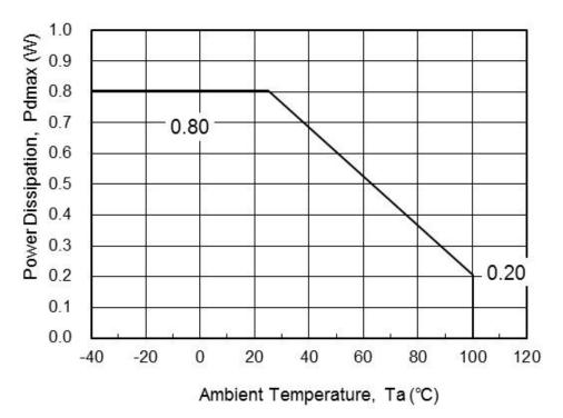
Figure 4. Pdmax vs T<sub>A</sub>
