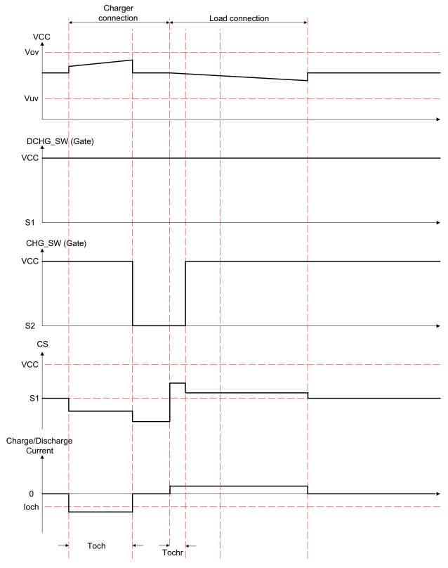
Figure 9. Charge Over-current Detection
