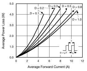
Fig. 2 - Forward Power Loss Characteristics
