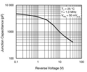
Fig. 5 - Typical Junction Capacitance
