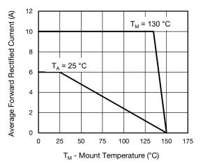
Fig. 1 - Maximum Forward Current Derating Curve Notes
