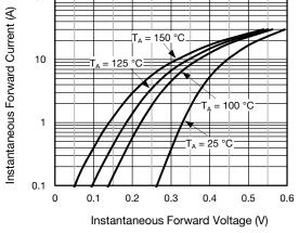
Fig. 3 - Typical Instantaneous Forward Characteristics
