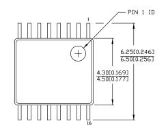
DIMENSIONS IN MMCINCHES)  $\frac{\text{MIN.}}{\text{MAX.}}$  REFERENCE JEDEC MO-153
