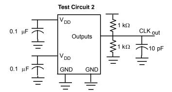
Test Circuit for  $t_8$ , Output slew rate on -1H, -5H device
