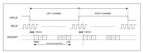
Figure 10 12S Justified Audio Interface (assuming n-bit word length)
