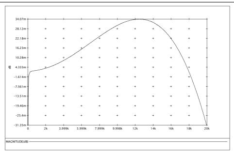
Figure 12 ADC Pass Band Frequency Response up to fs/2 (Sample rate, fs = 48kHz)
