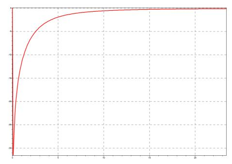
Figure 13 ADC High Pass Filter Frequency Response (Sample rate, fs = 48kHz)
