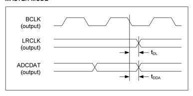
Figure 3 Audio Interface Timing - Master Mode
