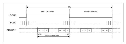
Figure 8 Right Justified Audio Interface (assuming n-bit word length)
