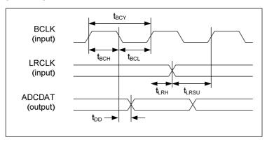
Figure 4 Audio Interface Timing - Slave Mode
