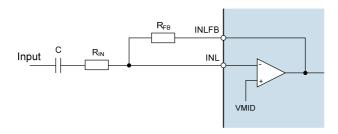
Figure 5 Input Signal Path Configuration
