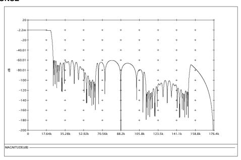
Figure 11 ADC Frequency Response up to  $4 \times fs$  (Sample rate, fs = 48kHz)
