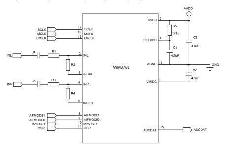
Figure 15 WM8788 Recommended External Components Diagram
