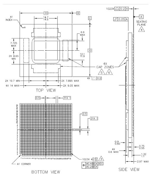
Figure 57. MPC8641D High-Head FC-CBGA Dimensions
