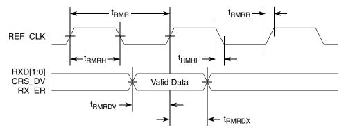
Figure 22. RMII Receive AC Timing Diagram
