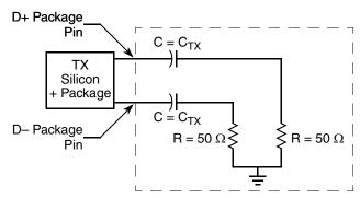
Figure 52. Compliance Test/Measurement Load
