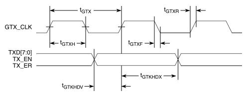
Figure 10. GMII Transmit AC Timing Diagram
