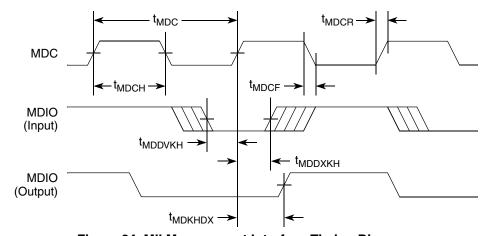
Figure 24. MII Management Interface Timing Diagram
