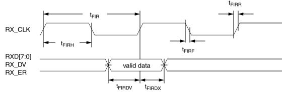
Figure 9. FIFO Receive AC Timing Diagram
