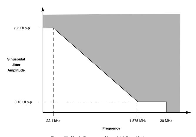
Figure 55. Single Frequency Sinusoidal Jitter Limits
