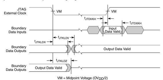
Figure 35. Boundary-Scan Timing Diagram
