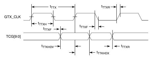
Figure 16. TBI Transmit AC Timing Diagram
