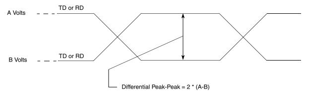
Figure 53. Differential Peak-Peak Voltage of Transmitter or Receiver
