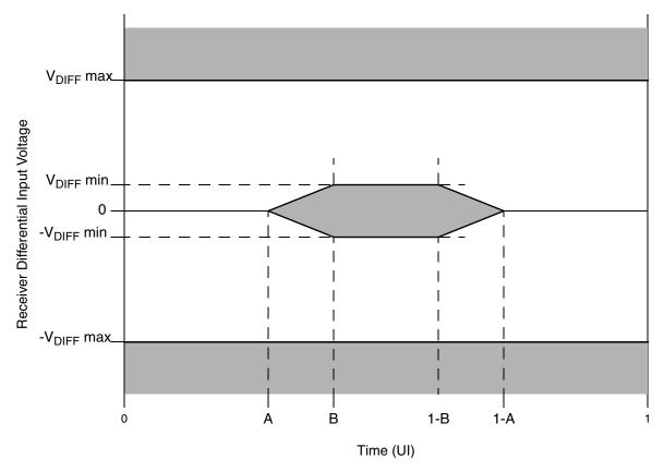
Figure 56. Receiver Input Compliance Mask
