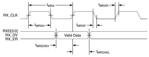
Figure 15. MII Receive AC Timing Diagram
