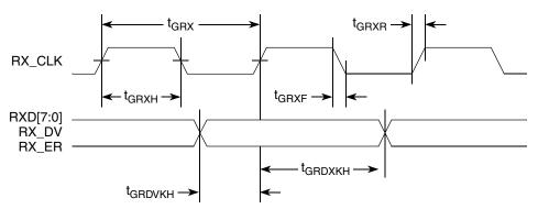
Figure 12. GMII Receive AC Timing Diagram
