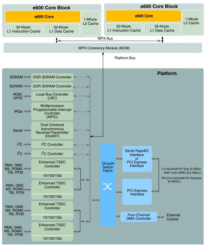
Figure 1. MPC8641 and MPC8641D
