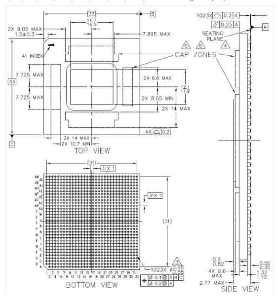
Figure 58. MPC8641D Lead-Free FC-CBGA Dimensions
