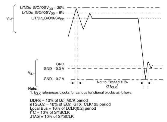
Figure 2. Overshoot/Undershoot Voltage for Dn\_M/O/L/TV<sub>IN</sub>
