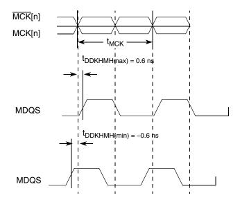
Figure 5. Timing Diagram for tDDKHMH
