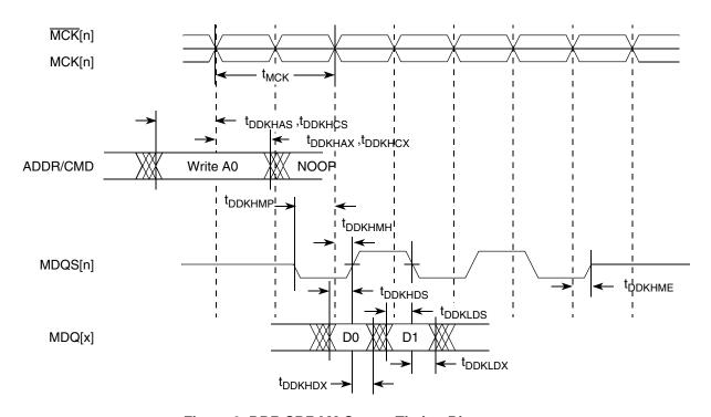
Figure 6. DDR SDRAM Output Timing Diagram
