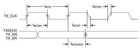
Figure 13. MII Transmit AC Timing Diagram
