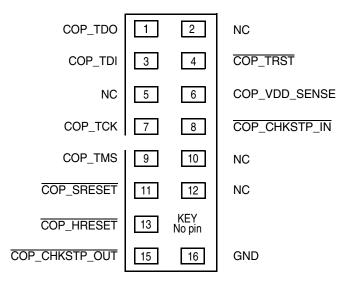
Figure 67. COP Connector Physical Pinout
