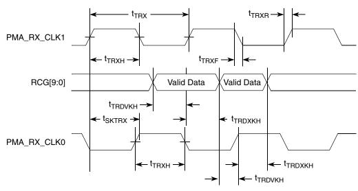
Figure 17. TBI Receive AC Timing Diagram
