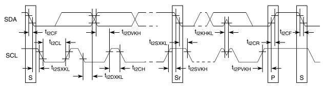
Figure 37. I<sup>2</sup>C Bus AC Timing Diagram
