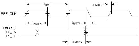
Figure 20. RMII Transmit AC Timing Diagram
