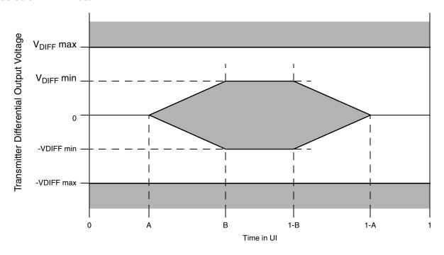
Figure 54. Transmitter Output Compliance Mask
