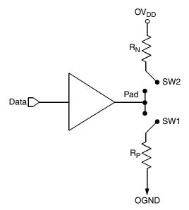
Figure 66. Driver Impedance Measurement
