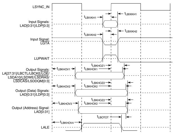
Figure 26. Local Bus Signals (PLL Enabled)
