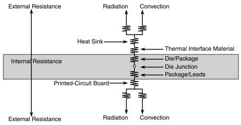
(Note the internal versus external package resistance.)
